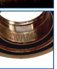
Marks on the clutch disc e.g. on the clutch disc retainer plate
