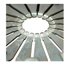
Pressure plate diaphragm finger tips, prematurely worn
