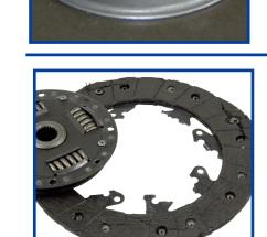
Clutch disc facing segments broken
