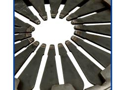
Clutch lever or diaphragm finger tips, bent or broken Note: The height difference of the diaphragm finger tips can only be measured when installed
