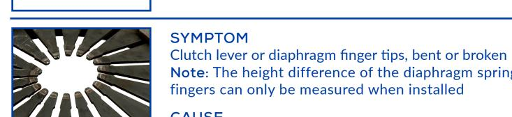
Note: The height difference of the diaphragm spring fingers can only be measured when installed
