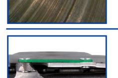
Tangential strap on clutch pressure plate bent or broken
