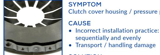
Clutch cover housing / pressure plate distorted
