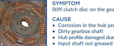
Stiff clutch disc on the gearbox input shaft
