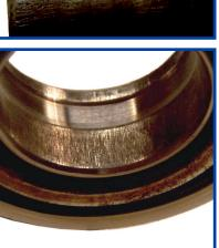
No grease or incorrect grade of grease
