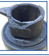
Gearbox guide tube worn / scoring marks on the bearing (inner diameter)
