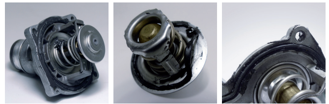
Figure 1: Thermostats with additional sealing compound
