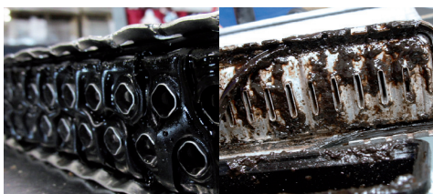
Figure 1: Rubber seals degraded by oil
