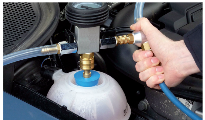
Figure 3: A vacuum is created in the system by means of the Venturi effect.
