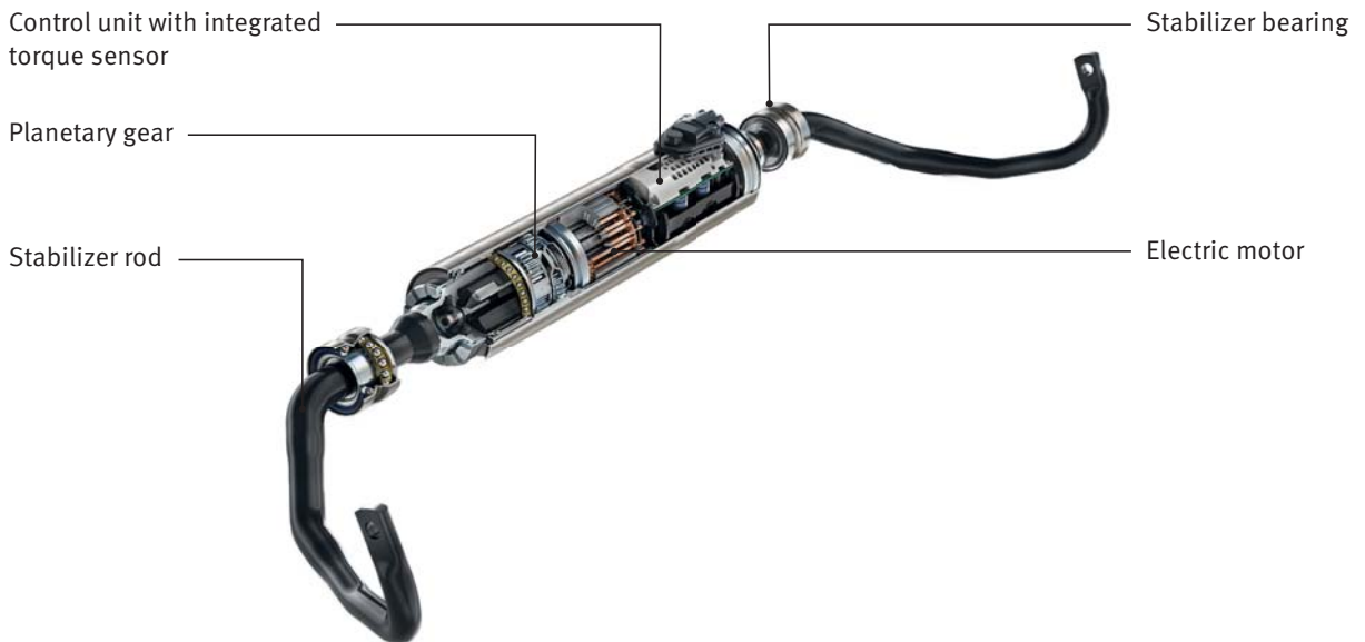
Electromechanical roll stabilizer
