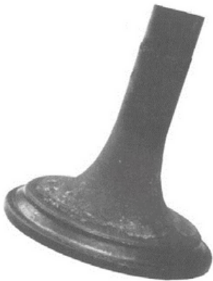
Exhaust Valve Face Wear
