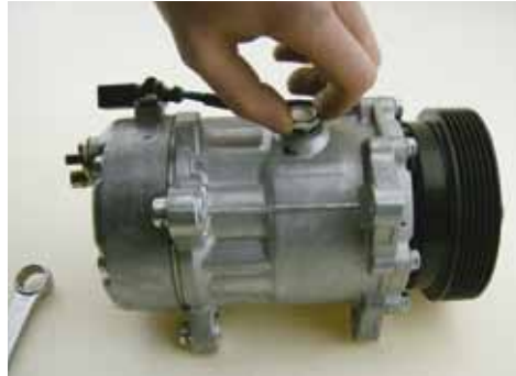
2. Turn out drain screw completely
