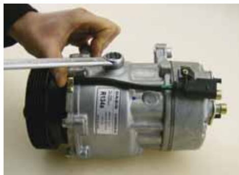
8. Tighten drain screw again
