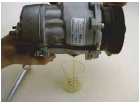
4. Exhaust compressor completely, turn clutch therefore
