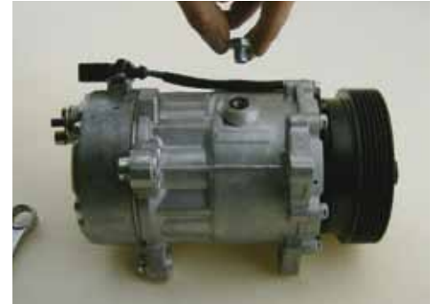
3. Remove drain screw
