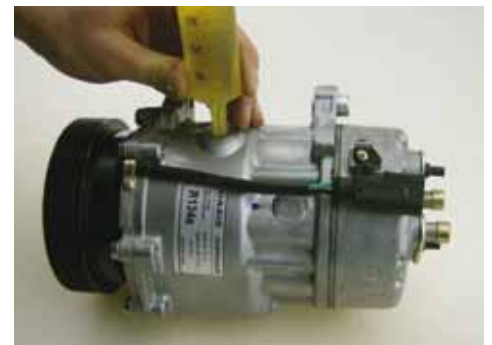
6. Adjust oil quantity according to manufacturer's advise
