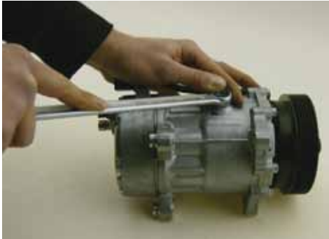
1. Loosen drain screw for oil carefully
